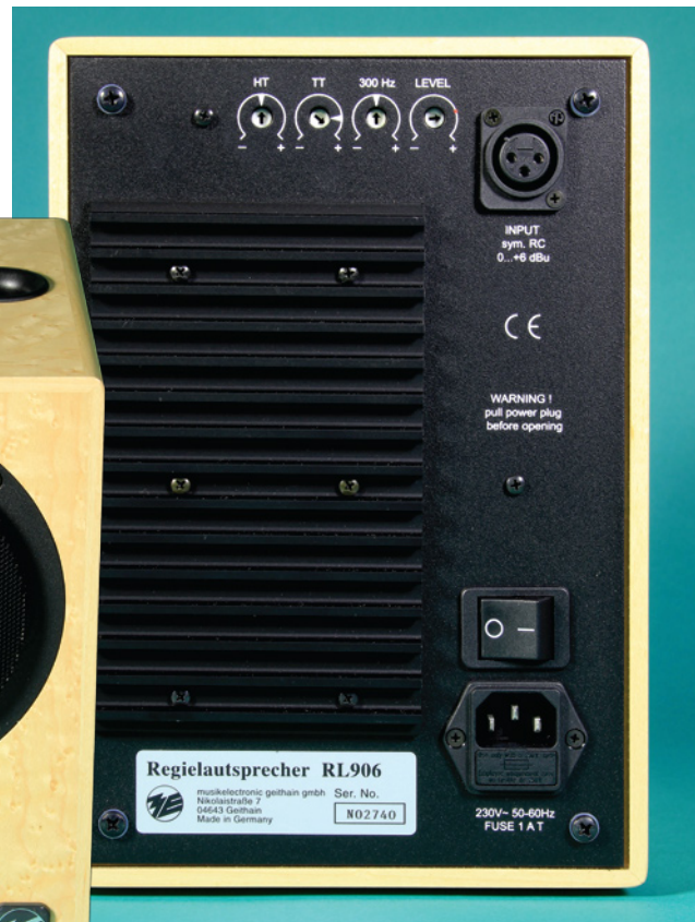
The RL906's rear panel houses the audio and power inputs, as well as EQ and level trim controls.
