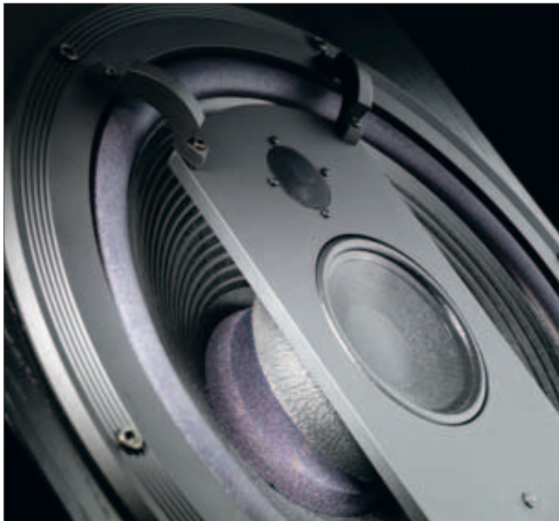
Free air: For achieving the purest sound, the midrange is free-air mounted into the baffle – a ring on the back with adjusted muffle inhibits an acoustic short.
