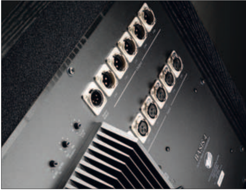
Bass manager: The Basis 4 K subwoofer fishes out bass parts from every surround channel separately – which is important for sound studios. Moreover, it has a classic LFE input.
