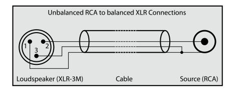
To carry the signal connect the XLR socket of the speaker to your signal source.
