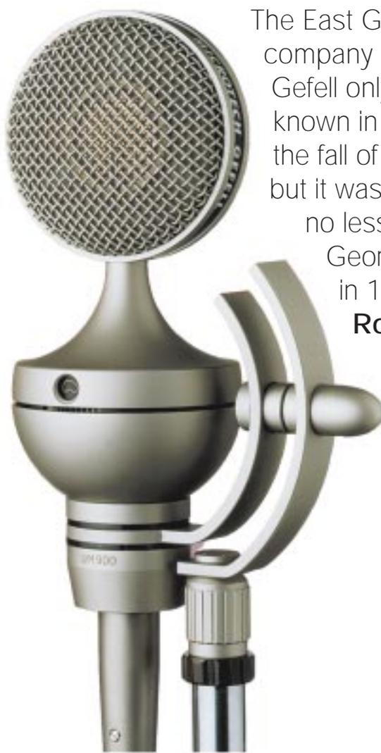
bracket, and by the polar pattern selector. This six-position rotary thumb switch rotates without end-stops and offers omni, sub-cardioid, cardioid, hypercardioid, figure-of-eight, and cardioid again — five different patterns. Since the sixth switch position is available, it might have been nice if the second cardioid pattern had offered a reverse-facing facility — like the Neumann
