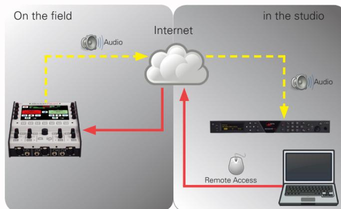
With AETA Remote Access feature, you can control all the parameters of your codecs remotely and in real time via the Internet, including via 4G mobile networks.
